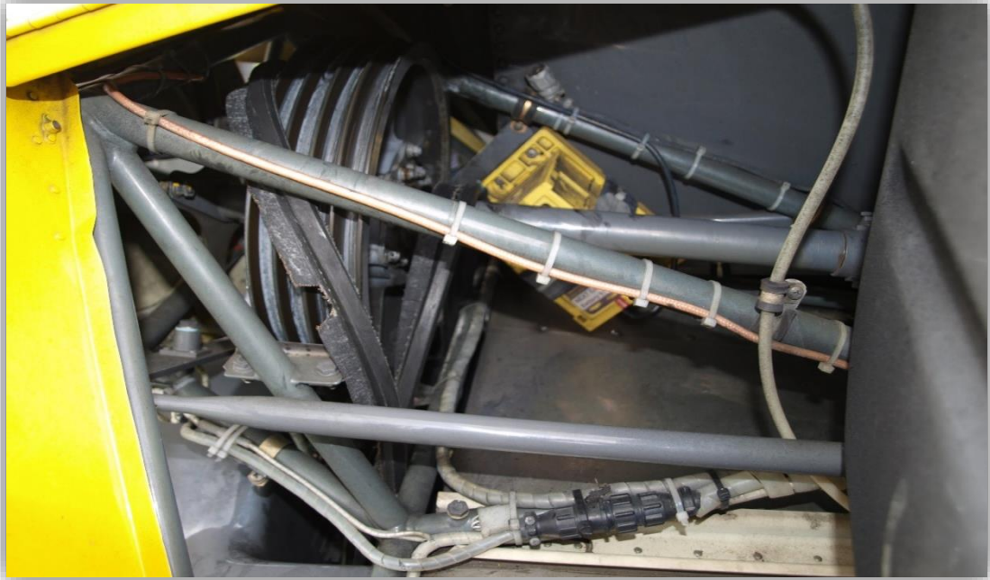
Fig. 3: The damaged front double V-belt in the engineering compartment
