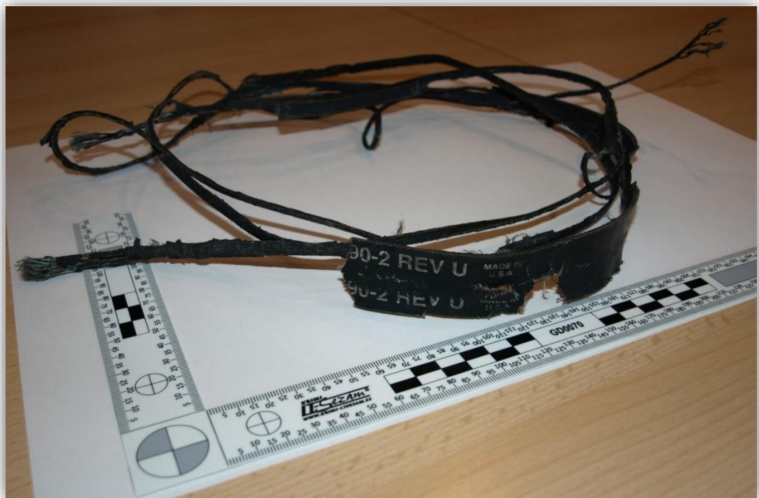
Fig. 2: The damaged rear double V-belt
