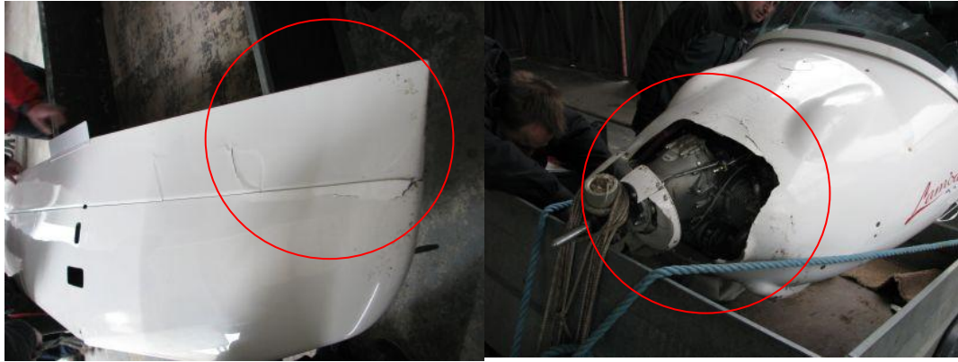
Damaged of horizontal tail plane and engine cowling
