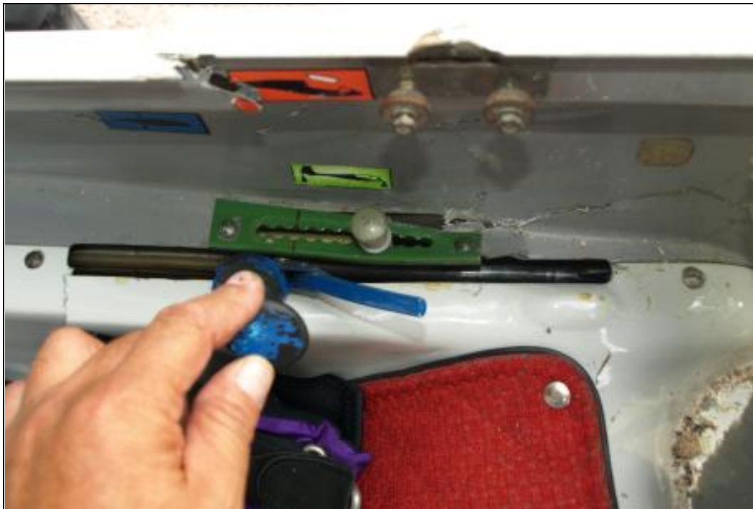
Position of stick to command air brakes and lengthwise balance
