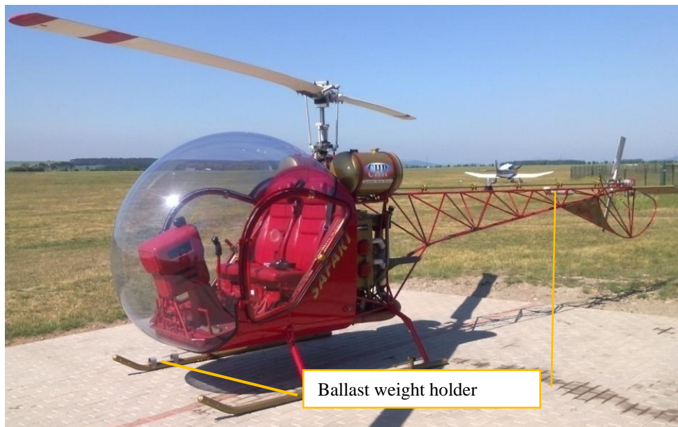
Fig. 3: Overall view of the Safari helicopter and ballast weight holder
