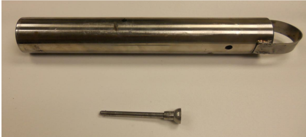
Fig. 7: Usual design of weight with locking pin (illustrative photo)
