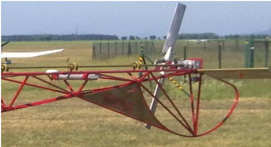
Fig. 6: Placement of ballast weight when occupied by two people
