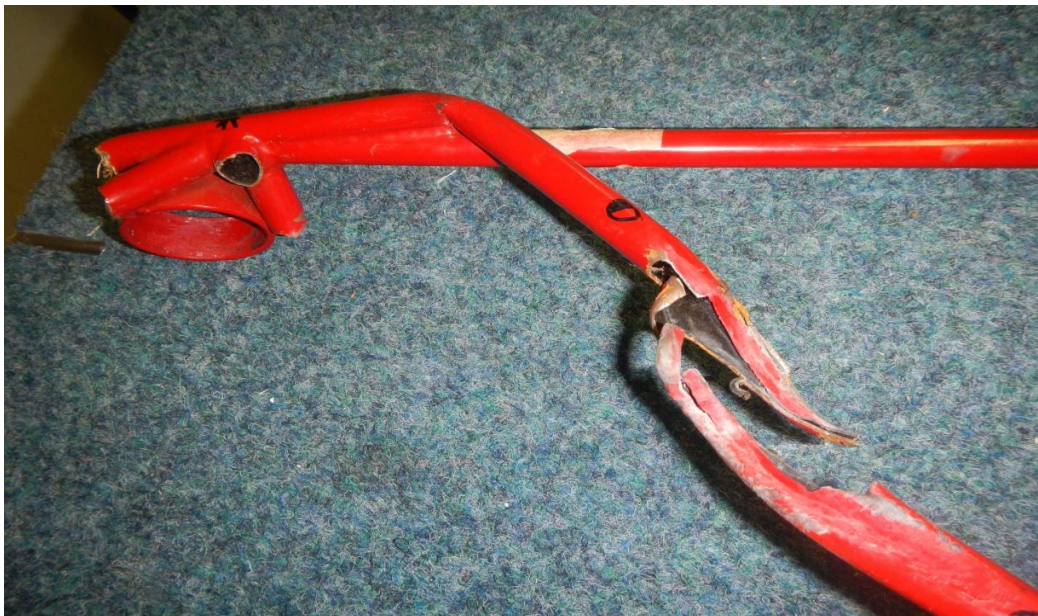
Fig. 8: Holder of the ballast weight on the right side of the tail beam
