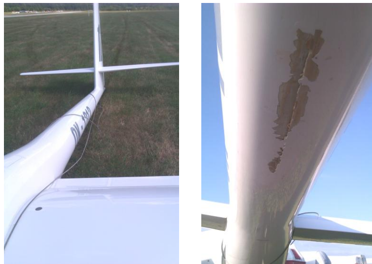
Figure 1 Status of the LAK 12 fuselage after the collision.
