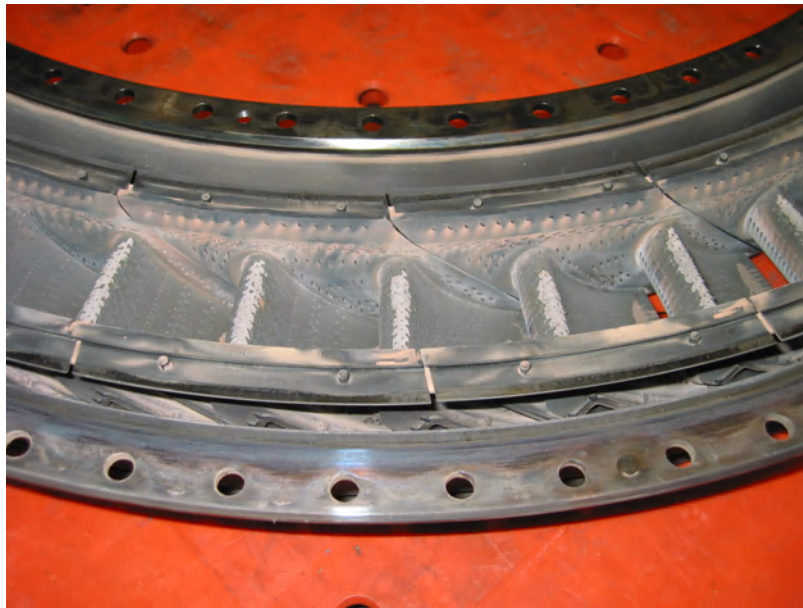
Fig. 3 Deposit of abrasion dust on high-pressure turbine stator blades
