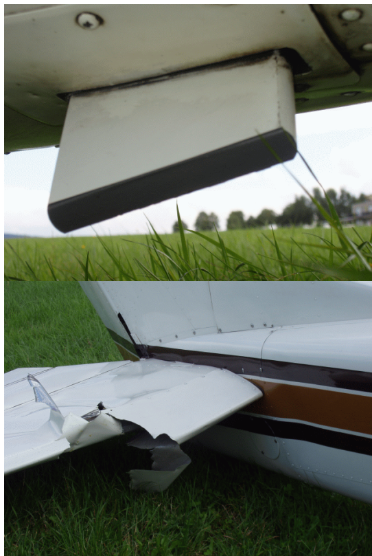
Pic.No 1- leg broke off, 95 mm away from its fixation
