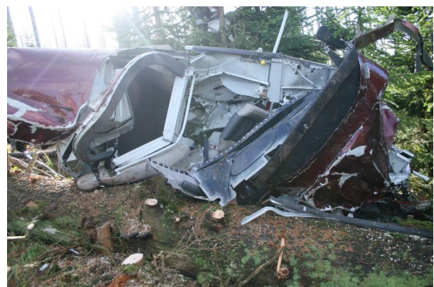
Closeup view of the deformed cockpit
