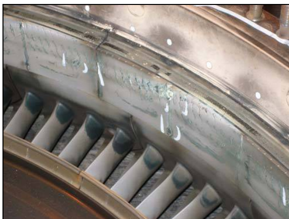
Fig 7 – Severe burning to a couple of HPT Shrouds (removal cause)
