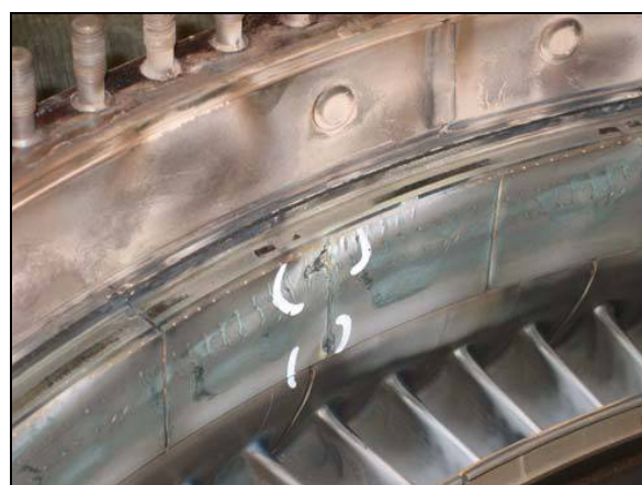
Fig 8 – Burning to more HPT Shrouds. 100% are likely to scrap.
