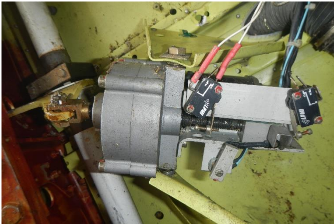
Flap power control
