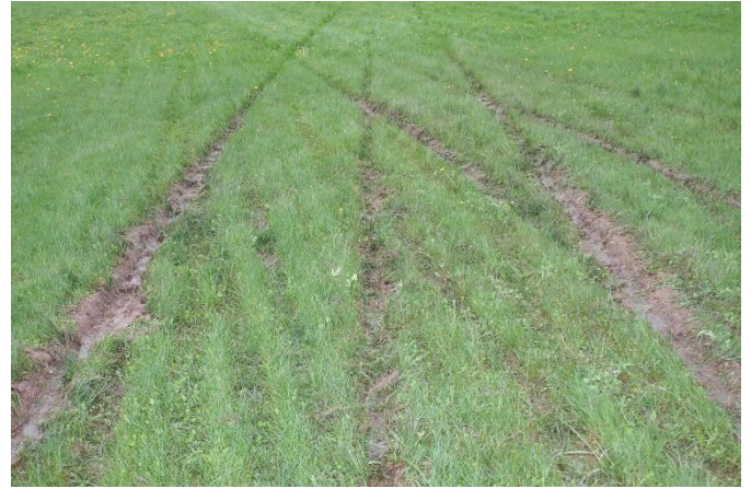
Tracks of landing gear wheels on muddy RWY
