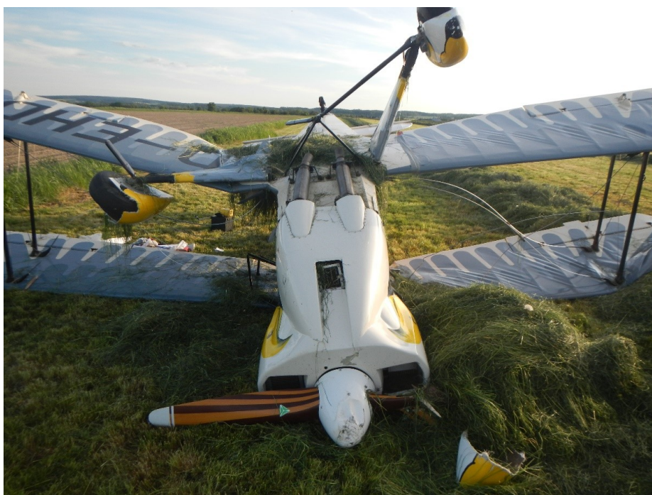
Fig. 6 – Extent of damage to the CASA 1.131-E aircraft.
