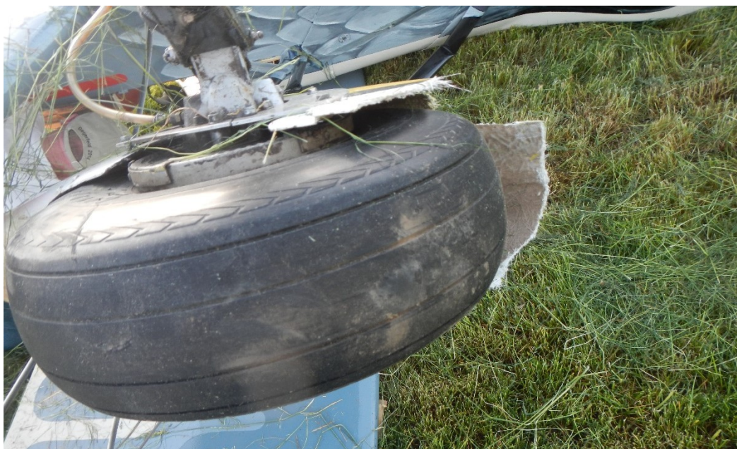
Fig. 4 – Traces of soil on the left gear wheel and broken streamline fairing of the wheel after running into a trench on the gliding strip.
