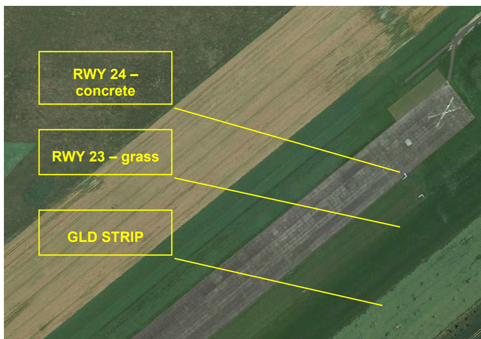
Fig. 15 – Visual markings of RWY 24 and GLD STRIP non-compliant with the requirements of Rule L 14 Aerodromes and RWY 23.
