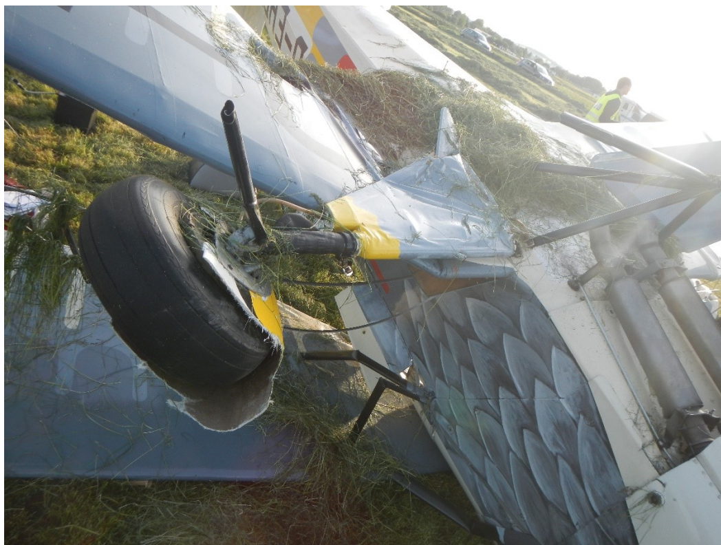
Fig. 12 – Damaged undercarriage, broken left wheel leg with a damaged wheel streamline fairing. Broken upper wing struts can be seen in the middle of the picture.
