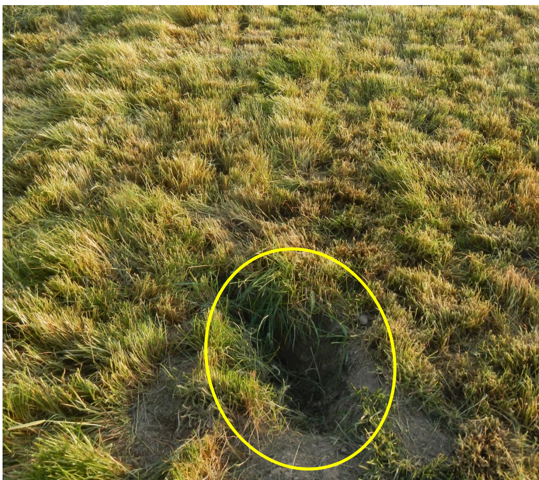
Fig. 3 – Trench in the surface of the gliding strip into which the left gear wheel ran.
