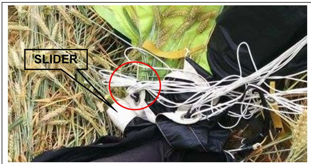
Fig. 4 The knot in the main parachute lines
